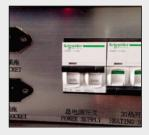
Separate the machine power and heating power to avoid huge current or electromagnetic wave disturb. Use SCHNEIDER switch.
