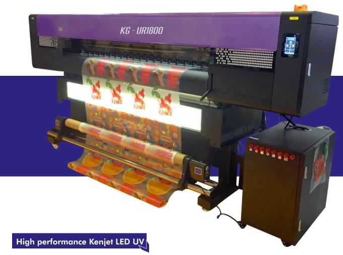
LED UV has the capability to be leading inkjet technology in the future. LESs produce very little heat which means they Can work with heat-sensitive media. They consume far less energy than conventional UV lamps and last up to ten times Longer. Above all they are much kinder to the Environment- A concern for printer operators and their alike.
