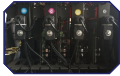
Electronic Sub-Tank System
