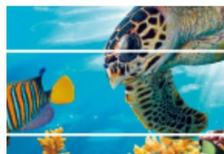
Gap/White streaks (Excessive feeding amount)
