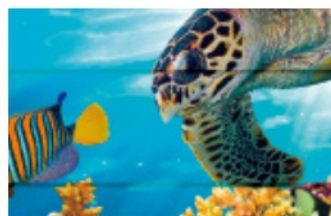
Overlap/Black streaks (Insufficient feeding amount)
