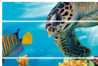
Gap/White streaks (Excessive feeding amount)
