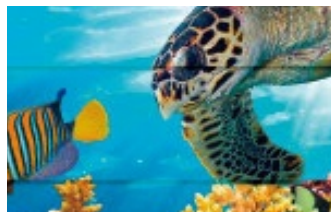
Overlap/Black streaks (Insufficient feeding amount)
