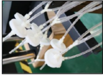
The Automatic Cleaning Assembly adds a Single-way Valve to Increase the Stability of the ink supply
